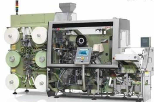
Example of a C-24E tea-packaging automatic machine [1]
