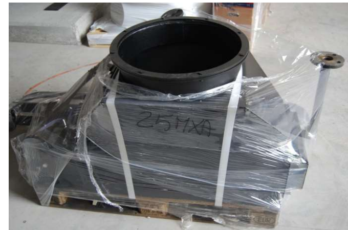
Economizer on flue gases (+ 3-4% efficiency increase)
