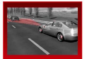
Radar-based driver assist systems can enhance the driving experience and, when combined with advanced electronic stability control brake systems, they can enable collision avoidance and mitigation.
